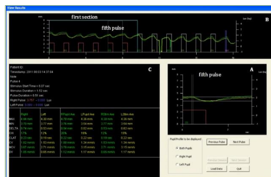
Figure 19 – The View Result GUI. The entire pupil profile (and stimulus waveform) is displayed in B. Pulse can be individually inspected in A. Pupil variables (belonging to that specific pulse in A) are reported in C. In this example, the fifth pulse of the first section has been selected in the display
