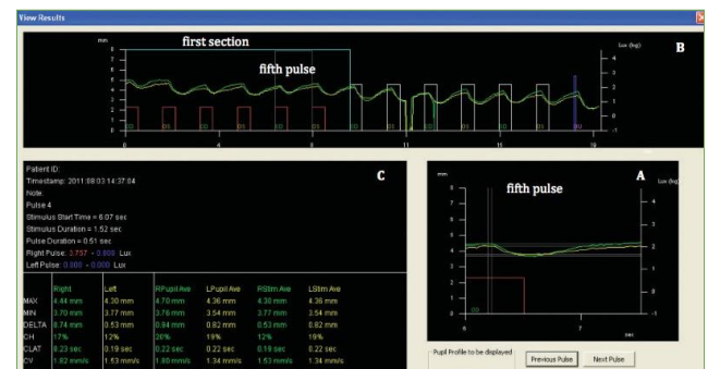
Figure 22– The View Result GUI. The entire pupil profile (and stimulus waveform) is displayed in B. Pulse can be individually inspected in A. Pupil variables (belonging to that specific pulse in A) are reported in C. In this example, the 5th pulse as the first section has been selected in the displayed
